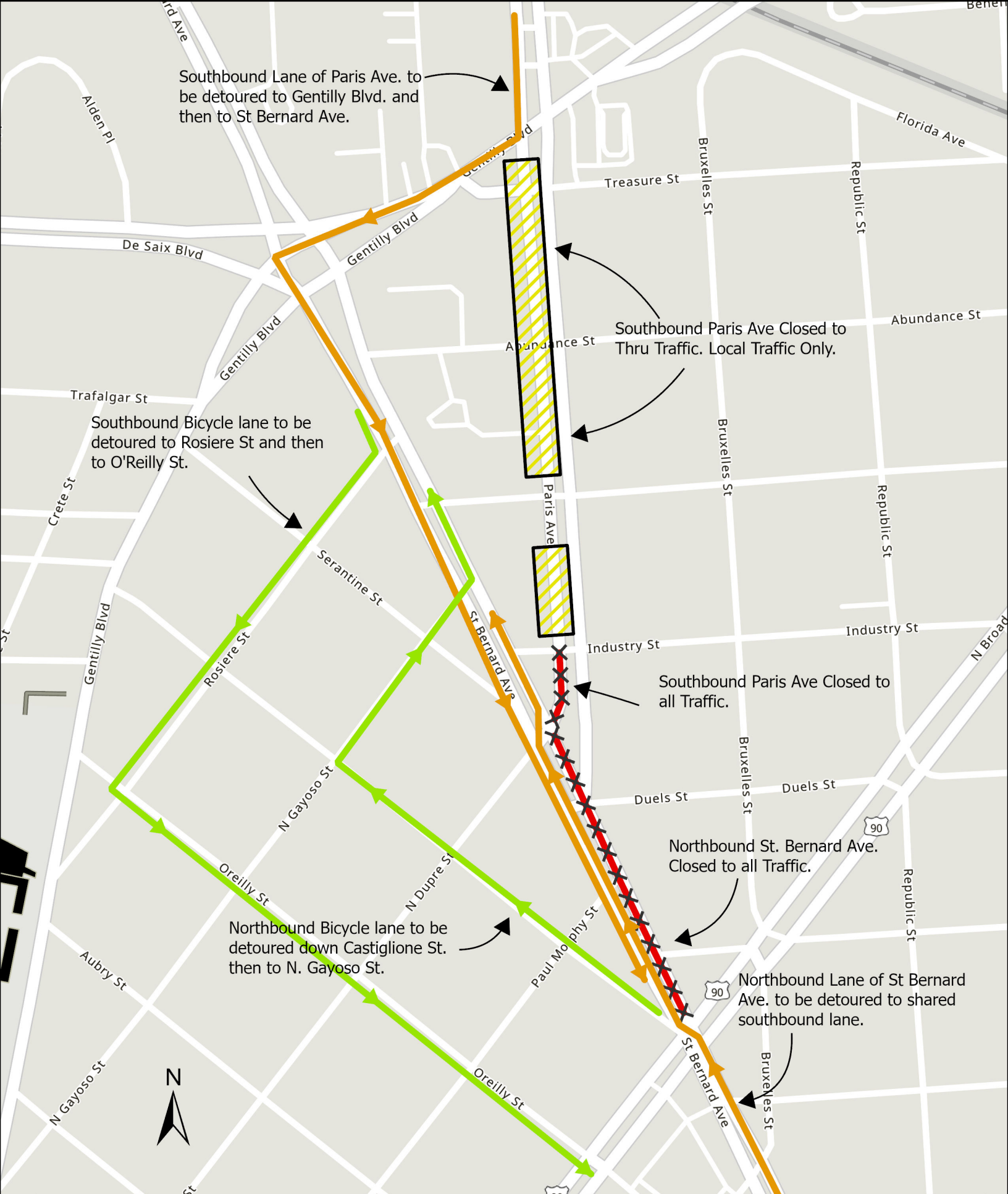
St. Bernard Ave. and N. Broad St. Temporary Traffic Flow
